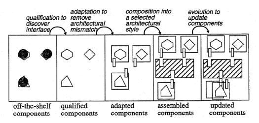
Figure 1: Model for architectural assembly of components.
